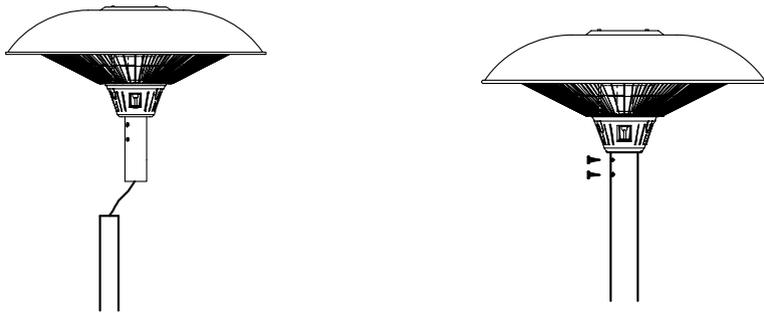
Step 7: Fix the power cable on to the base by using the supplied 4 pcs M4 Screws
