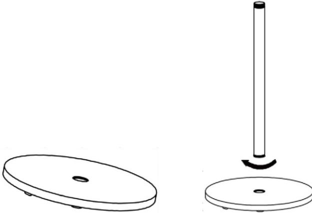
Step 2: Feed the Power Cable through the base and the bottom tube, and pull through around 2m of the power cable.
