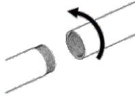
Step 4: Raise the Top tube to the desired height by screwing the fixation dial.
