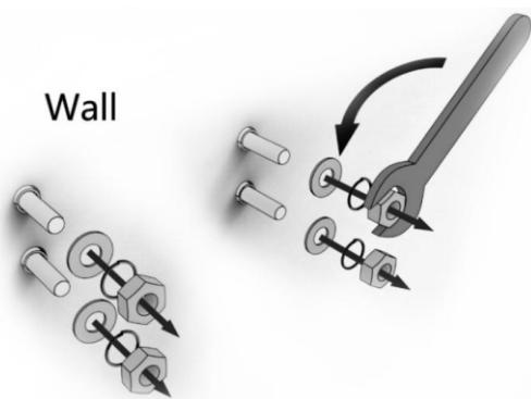
Step 3: Install the heater on the wall, then replace the spring lock washers, plain washers and nuts then tighten using the spanner.
