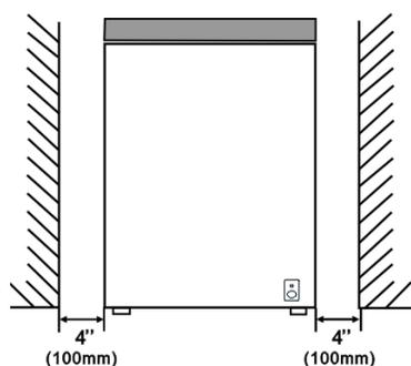
Make sure that sufficient room is provided around the appliance to ensure free air circulation. Ideally, A space of no less than 10cm must be left around the freezer, and ensure you allow gaps as shown.
