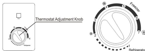
The inside temperature of freezer is regulated by thermostat adjustment knob.
