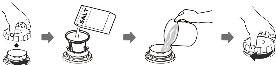
1. Remove the basket and unscrew the reservoir cap.
