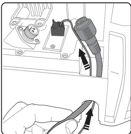
Feed the power lead up through the other side of the base station
